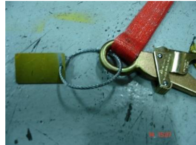
Figure 11: Lanyard showing Colour Coding Tag – opposite side of identifier
