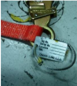
Figure 10: Lanyard showing unique identifier
